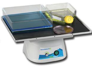
The Orbi-Blotter features a gentle orbital motion with speed control down to as little as 3 rpm, making it the ideal orbital choice for low speed applications, such as blotting, washing, staining/destaining, etc. A large 14x12 in. platform is included along with a non-slip rubber mat for holding trays, dishes, plates, flasks and other flat bottomed vessels. An optional stacking platform is also available for protocols requiring an increased work surface.
